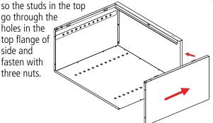
**6.** Attach the sill (Ref. No. 6) to the sides. Place nuts loosely on each of the studs and slide the ends of the sill into the slots on both sides of the unit. Then, securely tighten the nuts.
