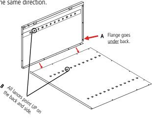
**4.** Attach the top (Ref. No. 5) to the unit by sliding the outer flange over the back of the unit and the side flange to the side panel on the unit. The threaded studs should go
