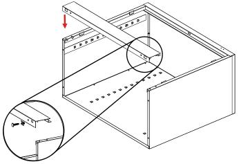
**7.** Place the rear flange of the bottom (Ref. No. 9) into the bottom lances of the back. The flange with two holes should face the front, hanging over the sill. Insert bolts through the bottom and sill with the head facing the front of the unit. Secure with two nuts.
