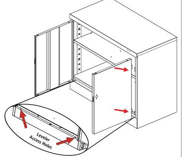
**12.** The cabinet must be level in order for the doors to close properly. Levelers may be adjusted by placing the nut driver through the hole in each end of the sill and adjusting the leveling screw.
